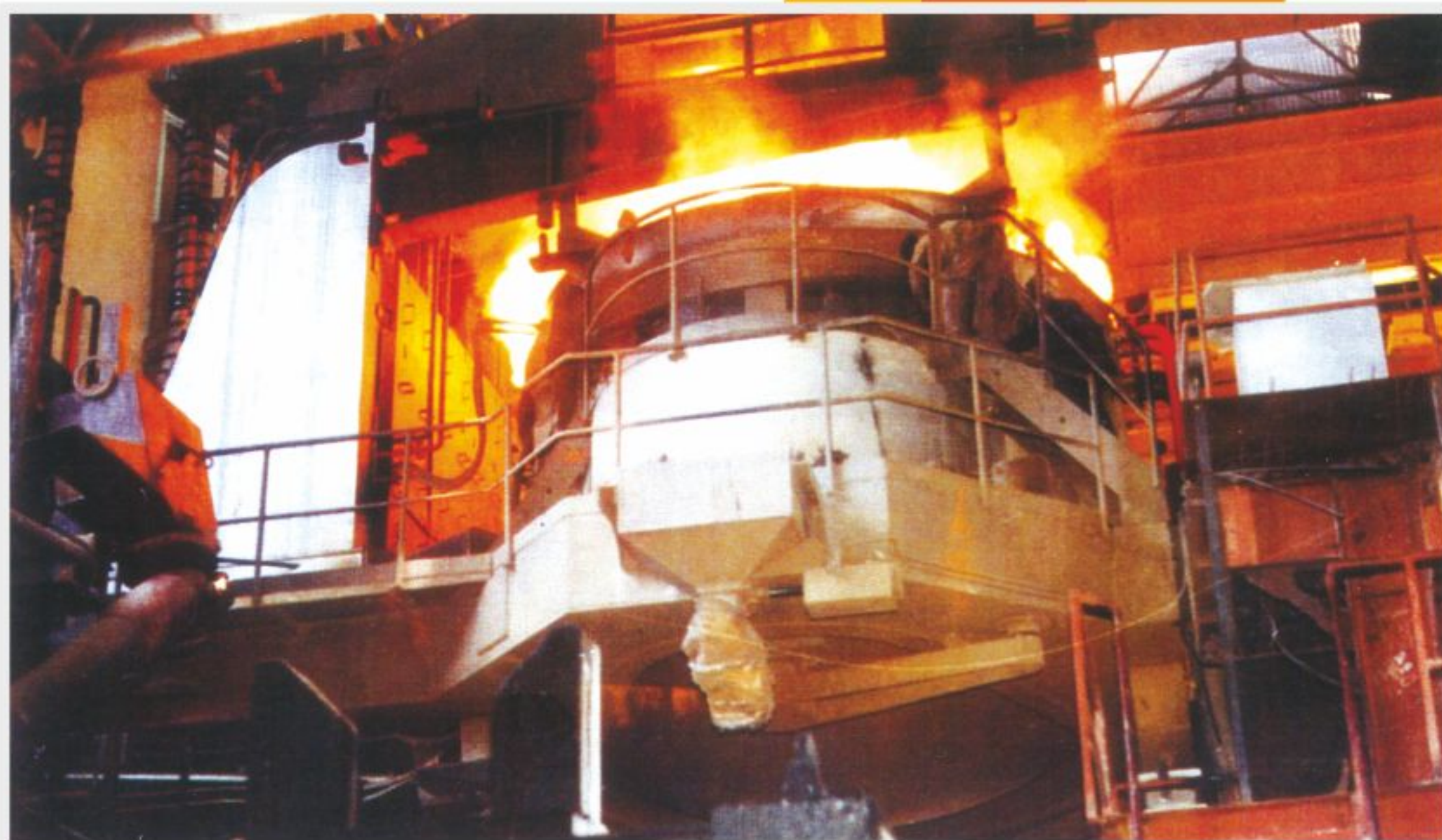
45 Tonne, UHP 36 MVA Arc Furnace type AL-460
